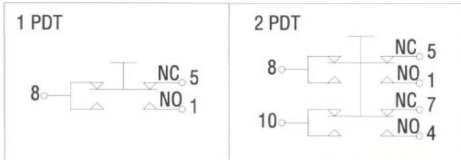
Form "C" Switch Circuits
