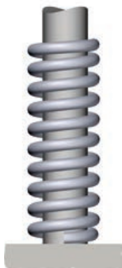
2. Not ground with internal location
